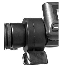
The throttle mechanism allows to activate pull power from a stop, and inexperienced users should take extra care when first applying the throttle. We recommend beginning the ride with pedaling first and then applying the throttle. Always be aware of your surroundings. Do not use the throttle unless you are ready to ride. As a precaution, turn the LCD off after riding to avoid accidental activating of the throttle or PAS.
